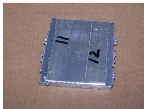
Fig. 3 Typical burrs generated during the experiments
